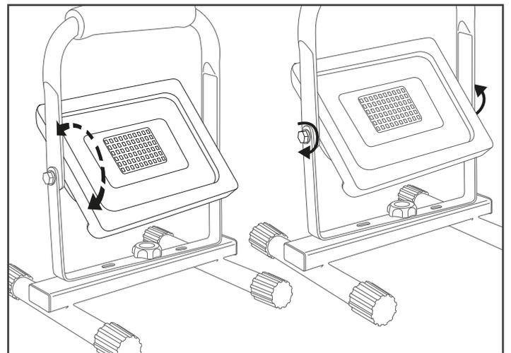
Floodlight has a vertical rotation of 270°, ensure cable does not tangle with the bracket. Periodically check the bolt and tighten if needed as this will become loose over time.
