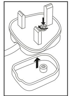
Replace cover and tighten screw to secure. Plug IP20 and should be used in dry locations.
