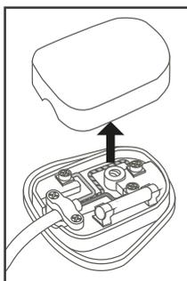
Ensure plug has cooled. Loosen screw and remove plug cover.
