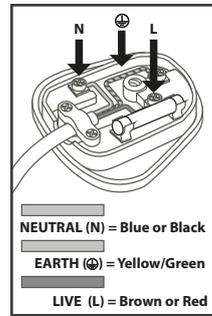
Ensure wires are securely attached with no loose bare wires. Product requires Earthing.
