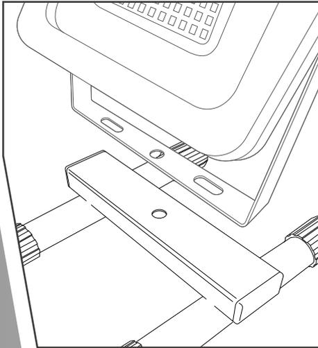
Position Floodlight bracket over Base bracket
