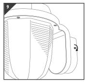
Secure fitting to bracket, do not over tighten the lug screws.
