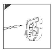
Ensure product is located in the correct location and mark the surface
