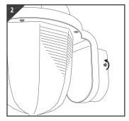
Slacken 2 lug screws from the fitting. Separate the mounting bracket from the fitting and wiring
