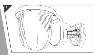
Place terminal block onto the securing pegs as the fitting is placed onto the mount bracket
