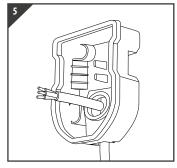
Thread the supply cable into the mount bracket before securing
