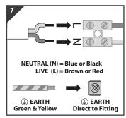
Insert correct supply (H05RN-F 1.0mm2 core cable) into terminal block, tighten all screws in block. Product MUST be earthed.
