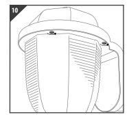
Hold light fitting casing whilst removal. Unscrew 4 securing screws and remove
