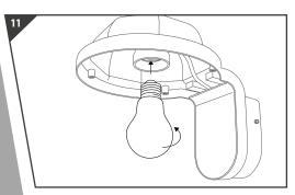
Insert correct wattage of GLS (E27 Cap) lamp into the fitting
