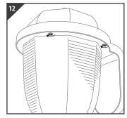
Return fitting casing, secure in place with all 4 screws, do not over tighten.
