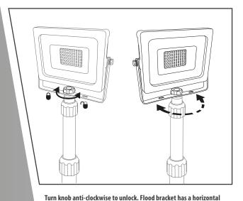
rotation of 360°, ensure cable does not tangle with the stand. Turn
