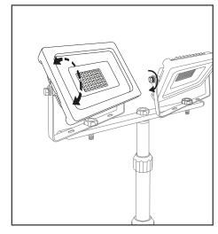
Floodlight has a vertical rotation of 360°, ensure cable does not tangle with the bracket. Periodically check the bolt and tighten if needed as this will become loose over time.
