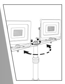
Turn knob anti-clockwise to unlock. Crossbar has a horizontal rotation of 360°, ensure cable does not tangle with the stand. Turn knob clockwise to lock in the desired location.
