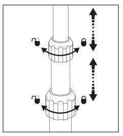
Loosen the compression nut by twisting anti-clockwise, extend the center pole and secure by retightening.
