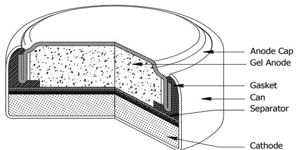
DESIGNED FOR USE ON CONTINUOUS LOW DRAIN
