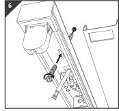
Secure the back panel to the surface
