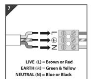
Insert supply cable into terminal block, tighten all screws in block. Product MUST be earthed
