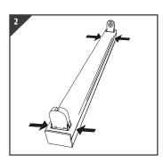
Remove the cover using a flat blunt instrument between cover and back panel, gently ease apart
