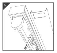
Thread the supply cable into the back panel before securing
