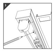
Ensure product is located in the correct location and mark the surface at each fixing hole
