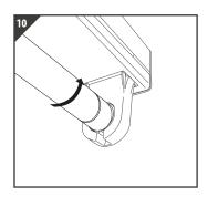
Rotate tube 90° in either direction to secure, do not exert too much force
