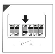
Switch OFF at mains supply before installing
