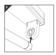
Insert the correct tube into the fitting ensuring pins slide smoothly into place
