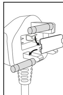
Remove 3-amp fuse and replace with an operational 3-amp fuse
