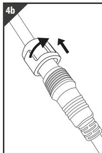
4b On the second string loosen the connecting cap in-between the plug and first light and separate
