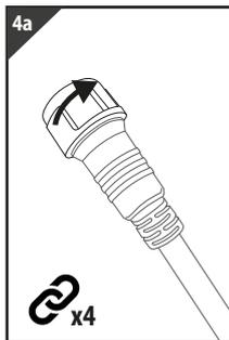
4a To link another set of string lights. On the first string remove the waterproof cover at the end of the cable
