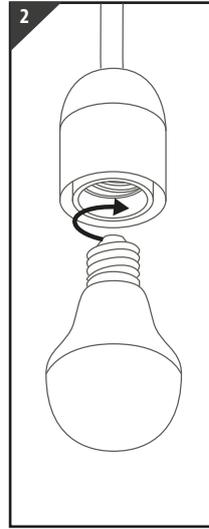
2 Screw in the E27/ES lamps into the screw in lampholders
