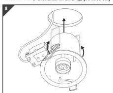
Push springs upwards against the body of the downlight and insert in the hole
