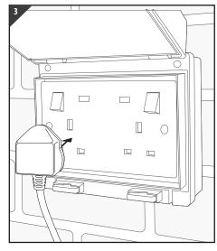
Ensure power source is dry (outdoor rated socket, IP rated box or Indoor location)
