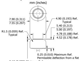
0.13 (0.005) Minimum Ref. (applies to top edge of gasket or edge of crimp, whichever is higher)
