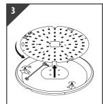
Loosen screws and twist to remove gear tray from the base, detach safety belt
