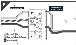
Press the individual terminal and insert the correct incoming supply before releasing the terminal to secure. The product MUST be earthed
