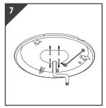
Install the fixing screws to the base Attach safety belt to gear tray
