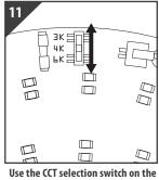
gear tray to select the desired colour temperature
