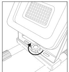
Tighten screw to lock into desired position
