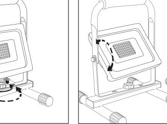
Floodlight has a vertical rotation of 270°, ensure cable does not tangle with the bracket. Periodically check the bolt and tighten if needed as this will become loose over time.
